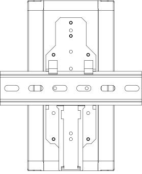
Figure 2.1. DIN Rail Mounting
